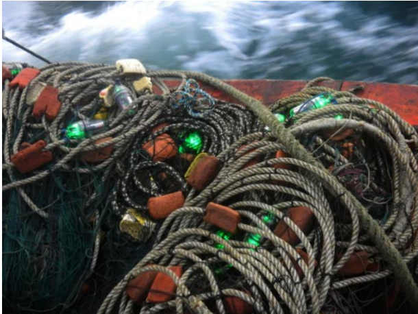
Slika 19. Led lampice montirane na mrežu stajaćicu (Izvor: https://marinemadness.blog/2019/12/18/using-led-lights-to-reduce-bycatch-in-gillnet-fisheries/ )
